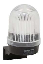
WERMA incandescent industrial tall signal beacon, 57mm, clear/white, permanent, IP65, bracket mount, 12-240 VAC/VDC. Requires incandescent bulb.
