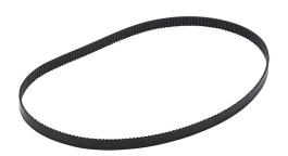
SureMotion timing belt, 0.08in MXL pitch, 1/4in wide, 212 tooth, 17in pitch length (circumference), polyurethane, polyester reinforced. Package of 3.
