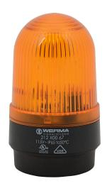
WERMA Xenon tube industrial tall signal beacon, 58mm, yellow, flashing strobe (0.75 Hz flash frequency), IP65, base mount, 115 VAC.
