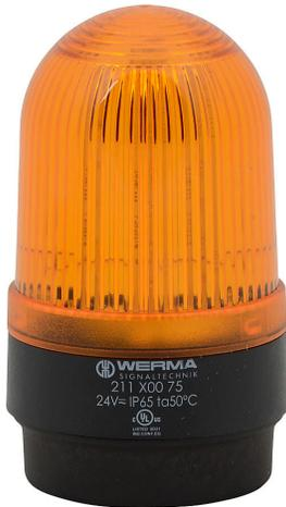
WERMA LED industrial tall signal beacon, 58mm, yellow, permanent, IP65, base mount, 24 VAC/VDC.
