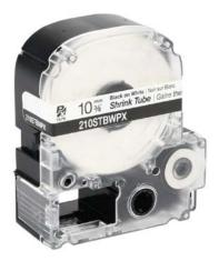
Epson LabelWorks PX series heat-shrink tube label cartridge, 10mm (3/8in) nominal diameter, 98in roll, black text, white background, polyolefin, 12-4 AWG. For use with Epson LabelWorks PX series label printers.
