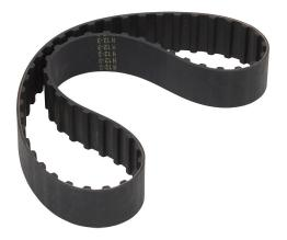
SureMotion timing belt, 3/8in L pitch, 1in wide, 56 tooth, 21in pitch length (circumference), neoprene, fiberglass reinforced.
