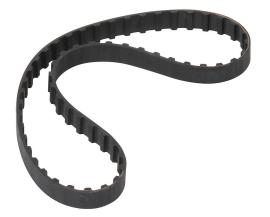
SureMotion timing belt, 3/8in L pitch, 1/2in wide, 56 tooth, 21in pitch length (circumference), neoprene, fiberglass reinforced.
