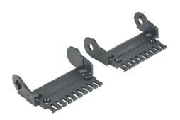
igus bracket, 0.98in inside height, 4.06in inside width, 90 to -48 deg pivoting, polyamide, black. For use with 2400 and 2500 series energy chain.
