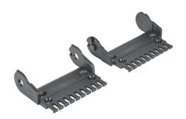
igus bracket, 0.98in inside height, 4.06in inside width, 90 deg locking and 0 deg locking, polyamide, black. For use with 2400 and 2500 series energy chain.
