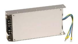
AutomationDirect EMI input filter, 230 VAC, 1-phase, 20A, panel mount, EMI/RFI filtering, drive rated, standard performance, screw terminals and ring terminals. For use with 1-phase AC drives.
