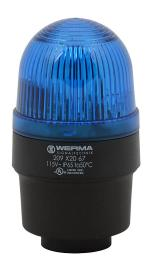
WERMA Xenon tube industrial signal beacon, 58mm, blue, flashing strobe (0.75 Hz flash frequency), IP65, tube mount, 115 VAC.
