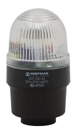
WERMA Xenon tube industrial signal beacon, 58mm, clear/white, flashing strobe (0.75 Hz flash frequency), IP65, tube mount, 24 VDC.
