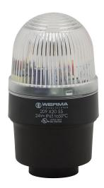
WERMA Xenon tube industrial signal beacon, 58mm, clear/white, flashing strobe (0.75 Hz flash frequency), IP65, tube mount, 24 VDC.
