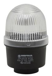
WERMA incandescent industrial signal beacon, 57mm, clear/ white, permanent, IP65, tube mount, 12-240 VAC/VDC. Requires incandescent bulb.
