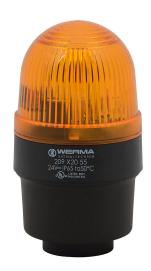
WERMA Xenon tube industrial signal beacon, 58mm, yellow, flashing strobe (0.75 Hz flash frequency), IP65, tube mount, 24 VDC.
