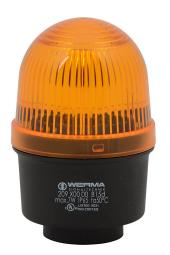
WERMA incandescent industrial signal beacon, 57mm, yellow, permanent, IP65, tube mount, 12-240 VAC/VDC. Requires incandescent bulb.
