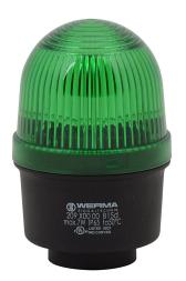
WERMA incandescent industrial signal beacon, 57mm, green, permanent, IP65, tube mount, 12-240 VAC/VDC. Requires incandescent bulb.
