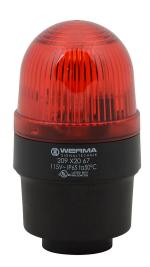
WERMA Xenon tube industrial signal beacon, 58mm, red, flashing strobe (0.75 Hz flash frequency), IP65, tube mount, 115 VAC.
