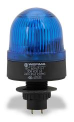
WERMA Xenon tube industrial signal beacon, 58mm, blue, flashing strobe (0.75 Hz flash frequency), IP65, 22.5mm panel mount, 24 VDC.
