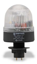
WERMA Xenon tube industrial signal beacon, 58mm, clear/white, flashing strobe (0.75 Hz flash frequency), IP65, 22.5mm panel mount, 24 VDC.
