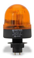
WERMA Xenon tube industrial signal beacon, 58mm, yellow, flashing strobe (0.75 Hz flash frequency), IP65, 22.5mm panel mount, 24 VDC.
