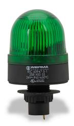
WERMA Xenon tube industrial signal beacon, 58mm, green, flashing strobe (0.75 Hz flash frequency), IP65, 22.5mm panel mount, 24 VDC.
