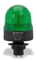
WERMA LED industrial signal beacon, 58mm, green, permanent, IP65, 22.5mm panel mount, 24 VAC/VDC.
