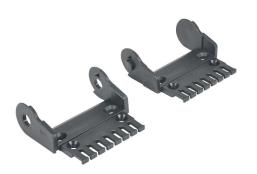
igus bracket, 0.98in inside height, 3.03in inside width, 90 to -48 deg pivoting, polyamide, black. For use with 2400 and 2500 series energy chain.
