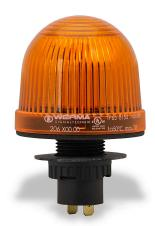
WERMA incandescent industrial signal beacon, 57mm, yellow, permanent, IP65, 22.5mm panel mount, 12-48 VAC/VDC. Requires incandescent bulb.
