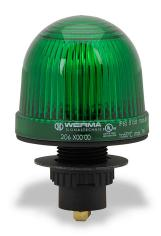
WERMA incandescent industrial signal beacon, 57mm, green, permanent, IP65, 22.5mm panel mount, 12-48 VAC/VDC. Requires incandescent bulb.
