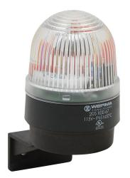
WERMA Xenon tube industrial signal beacon, 58mm, clear/white, flashing strobe (0.75 Hz flash frequency), IP65, bracket mount, 115 VAC.
