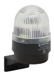
WERMA Xenon tube industrial signal beacon, 58mm, clear/white, flashing strobe (0.75 Hz flash frequency), IP65, bracket mount, 24 VDC.
