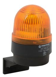
WERMA Xenon tube industrial signal beacon, 58mm, yellow, flashing strobe (0.75 Hz flash frequency), IP65, bracket mount, 115 VAC.
