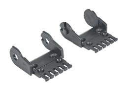
igus bracket, 0.98in inside height, 2.24in inside width, 90 deg locking and 0 deg locking, polyamide, black. For use with 2400 and 2500 series energy chain.
