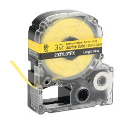
Epson LabelWorks PX series heat-shrink tube label cartridge, 3mm (1/8in) nominal diameter, 98in roll, black text, yellow background, polyolefin, 22-14 AWG. For use with Epson LabelWorks PX series label printers.
