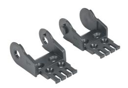
igus bracket, 0.98in inside height, 1.5in inside width, 90 to -48 deg pivoting, polyamide, black. For use with 2400 and 2500 series energy chain.
