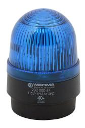
WERMA Xenon tube industrial signal beacon, 58mm, blue, flashing strobe (0.75 Hz flash frequency), IP65, base mount, 115 VAC.
