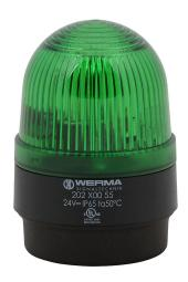
WERMA Xenon tube industrial signal beacon, 58mm, green, flashing strobe (0.75 Hz flash frequency), IP65, base mount, 24 VDC.
