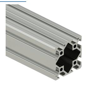
SureFrame 10 Series standard T-slotted rail, silver, 6063-T6 anodized aluminum alloy, cut to length, 2 x 2in profile, slot size 6.
