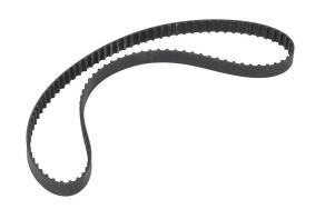
SureMotion timing belt, 1/5in XL pitch, 3/8in wide, 100 tooth, 20in pitch length (circumference), neoprene, fiberglass reinforced.
