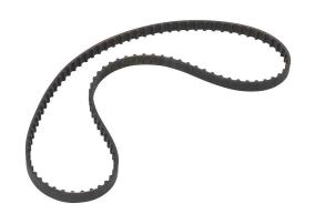
SureMotion timing belt, 1/5in XL pitch, 1/4in wide, 100 tooth, 20in pitch length (circumference), neoprene, fiberglass reinforced.
