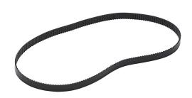
SureMotion timing belt, 0.08in MXL pitch, 1/4in wide, 200 tooth, 16in pitch length (circumference), polyurethane, polyester reinforced. Package of 3.
