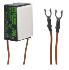
Murrelektronik universal surge suppressor, resistor-capacitor, 24-60 VAC/VDC, 1-phase, 0-60Hz, 15W, pigtail with spade connectors, adhesive foil and cable tie mount.
