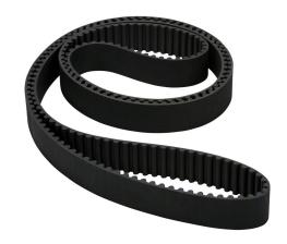
SureMotion timing belt, 8mm 8M pitch, 30mm wide, 250 tooth, 2000mm pitch length (circumference), neoprene, fiberglass reinforced.
