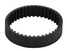
SureMotion timing belt, 5mm 5M pitch, 15mm wide, 40 tooth, 200mm pitch length (circumference), neoprene, fiberglass reinforced.
