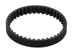
SureMotion timing belt, 5mm 5M pitch, 9mm wide, 40 tooth, 200mm pitch length (circumference), neoprene, fiberglass reinforced.
