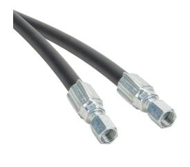
Gates ProFlex petroleum based hydraulic fluid hose assembly, synthetic rubber, braided steel wire reinforced, black, 1/4in inside diameter, 0.52in outside diameter, (2) -4 female straight JIC 37 deg fittings, 8ft working length.
