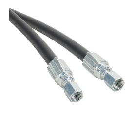
Gates ProFlex petroleum based hydraulic fluid hose assembly, synthetic rubber, braided steel wire reinforced, black, 1/4in inside diameter, 0.52in outside diameter, (2) -4 female straight JIC 37 deg fittings, 6ft working length.
