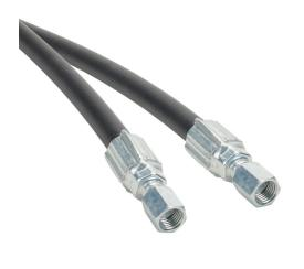
Gates ProFlex petroleum based hydraulic fluid hose assembly, synthetic rubber, braided steel wire reinforced, black, 1/4in inside diameter, 0.52in outside diameter, (2) -4 female straight JIC 37 deg fittings, 2ft working length.
