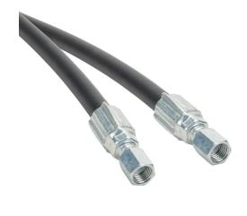
Gates ProFlex petroleum based hydraulic fluid hose assembly, synthetic rubber, braided steel wire reinforced, black, 1/4in inside diameter, 0.52in outside diameter, (2) -4 female straight JIC 37 deg fittings, 10ft working length.
