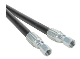
Gates MXT petroleum based hydraulic fluid hose assembly, synthetic rubber, braided steel wire reinforced, black, 1/4in inside diameter, 0.55in outside diameter, (2) -4 female straight JIC 37 deg fittings, 6ft working length.
