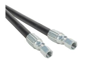
Gates MXT petroleum based hydraulic fluid hose assembly, synthetic rubber, braided steel wire reinforced, black, 1/4in inside diameter, 0.55in outside diameter, (2) -4 female straight JIC 37 deg fittings, 4ft working length.
