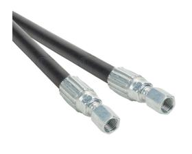
Gates MXT petroleum based hydraulic fluid hose assembly, synthetic rubber, braided steel wire reinforced, black, 1/4in inside diameter, 0.55in outside diameter, (2) -4 female straight JIC 37 deg fittings, 10ft working length.
