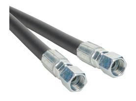
Gates ProFlex petroleum based hydraulic fluid hose assembly, synthetic rubber, braided steel wire reinforced, black, 1/2in inside diameter, 0.81in outside diameter, (2) -8 female straight JIC 37 deg fittings, 8ft working length.
