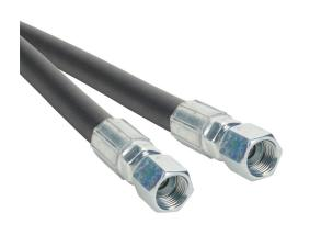
Gates ProFlex petroleum based hydraulic fluid hose assembly, synthetic rubber, braided steel wire reinforced, black, 1/2in inside diameter, 0.81in outside diameter, (2) -8 female straight JIC 37 deg fittings, 6ft working length.
